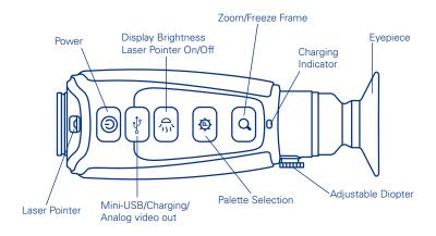
Power Button - The LSX-R has three power states: On, Off, and Auto Shutdown.
