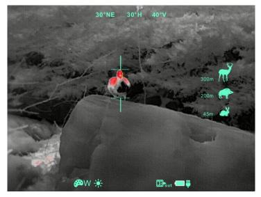
Fig. 6-7 Stadiametric rangefinder interface
