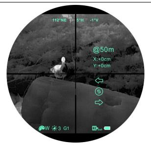
Fig. 6-6 Image calibration interface
