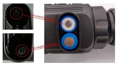
Fig. 8-1 Schematic diagram of battery installation
