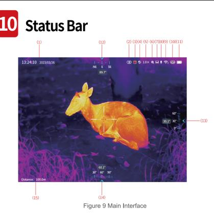
1.Time and date: display the current time and date. It can be modified in System Menu $\rightarrow$  System Settings $\rightarrow$  Time Settings.
