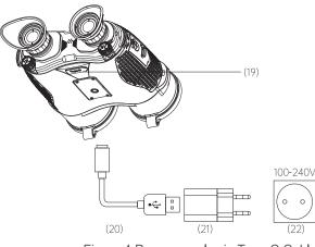
Figure 4 Power supply via Type-C Cable
