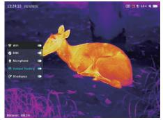
Figure 19 Hotspot Tracking 5.IR Enhance: short press the Menu button (4) to enable IR Enhance to present more details, disabled by default.
