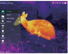
Figure 20 Display Menu 1.Screen Brightness: real-time adjustment on screen brightness adjustment, adjustment range 1-5, 3 by default. 2.Image Brightness: real-time adjustment on IR/NV image brightness, adjustment range 1-5, 3 by default, supported in IR or NV mode.
