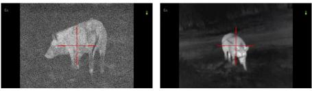
NUC'ing helps to improve the image quality when the image is degraded by various environmental factors. There are multiple NUC tables that span the full operating temperature range, and the scope automatically selects the optimum table based on its temperature.
