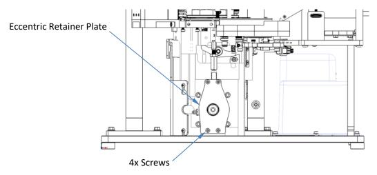
2. Remove Pin and slide out Swage Rod Assy.
