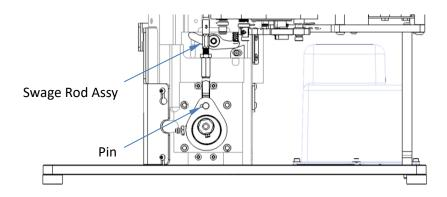
3. Replace Swage Rod Assy with SwageSense Assy. Secure with Pin.
