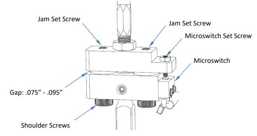
5. Tighten the Shoulder Screws evenly until desired gap is reached. Tighten two Jam Set Screws.
