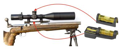
5) Once you are happy with the position of your riflescope, begin to torque down your rings in a criss-cross pattern, moving between screws and turning small amounts at a time. This will ensure that the riflescope does not shift position while tightening.
