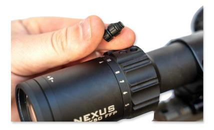
Your NEXUS will need to be zeroed after it has been fitted to your rifle. The first step is to remove your turrets and remove the zero stop mechanism to allow a full range of adjustment.
