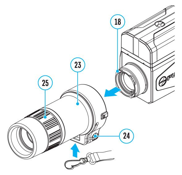
The **Pulsar 3x20 B monocular (23)** allows you to transform the device into a hand-held thermal imager with 3x magnification.
