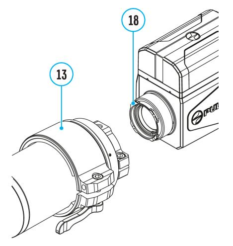
**1.** Remove the protective cover from the eyepiece of the thermal imaging module.
