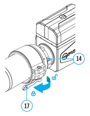
**1.** Loosen the screw (14) with an Allen key (S = 4mm).
