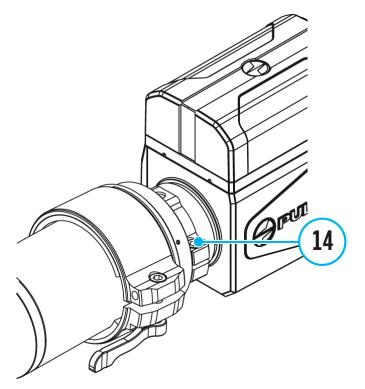
**5.** By tilting the thermal imaging module, align the center of the image in the eyepiece of the optical device with the auxiliary cross.
