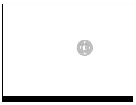
**Contrast**  $\mathbf{O}$  – press the **UP (5)/DOWN (7)** buttons to change the display contrast value from 0 to 20.
