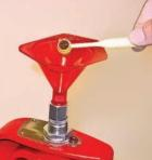
CAUTION After charging the case the only operation that should be done is to seat the bullet. Never try to seat a primer after powder has been added.
