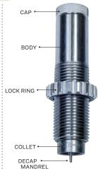
ADJUSTMENT FOR LEE PRESSES Screw sizing die in until it contacts the shell holder, plus one more turn (13/4 turns for Classic Series press owners).
